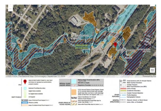
As you can see, the driveway, storm water run offs, new outlet intakes, retaining walls, portions of parking lots, as well as portions Building #2/4 &8 will all fall within that flood zone. And if this current floodplain were to be altered in any way, including impervious structures, & altered land use, it will also increase flooding potentials to neighboring parcels.
